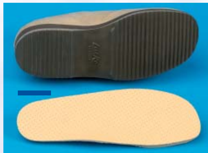
Fig. 1 Shape of the bottom of the stock ‘diabetic’ shoe under study, and the insole, respectively. Size 27.5cm French system. Bar indicates 5 cm distance.
